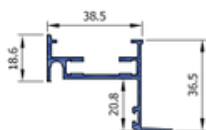
FG Sash Single Glazing CW3871
